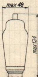
Abmessungen in mm; Dimensions en mm; Dimensiones in mm.
