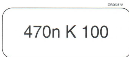
Fig.35 Example of marking for a capacitor with a body length of 10.0 or 12.5 mm.
