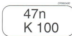
Fig.34 Example of marking for a capacitor with a body length \leq 7.5 mm.
