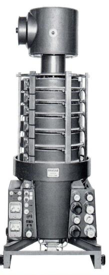
The PT 1001 is an 'S' band, water cooled, pulsed, 6 cavity klystron amplifier with electromagnetic focusing. Peak pulse powers of between 4 and 10 MW can be obtained with this tube which was designed for use in high power surveillance and air traffic control radar systems.
