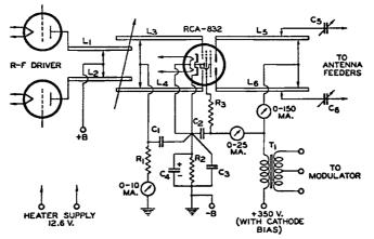
C1,C2,C3 = 500 MM C4=25 Uf, 200 VOLTS C5,C6 = 3 TO 35 UUF R1=10000 TO 20000 OHMS, I WATT R2 = 300 OHMS, 5 WATTS R3 = 7500 OHMS, 5 WATTS LI, L2 = DIMENSIONS DEPENDENT ON TYPE OF DRIVER TUBE; APPROX. SAME AS L5 L6.
