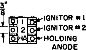
VIEW SHOWING IGNITOR AND HOLDING-ANODE TERMINALS
