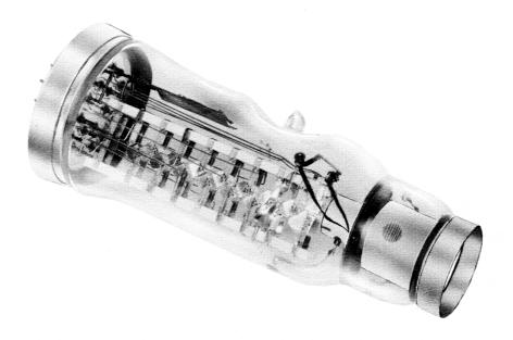
The Multiplier Phototube type 6836 is a 16-stage multiplier of the end-window type having an S-1 spectral sensitivity characteristic. To minimize cathode noise the active cathode in this tube is reduced to a central area of approximately 1/8-inch diameter. The tube is capable of detecting and measuring extremely weak sources of infrared radiation and will
