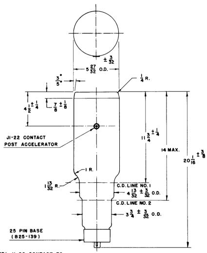
NOTE: JI-22 CONTACT TO ALIGN WITH BASE KEY + 10\*
