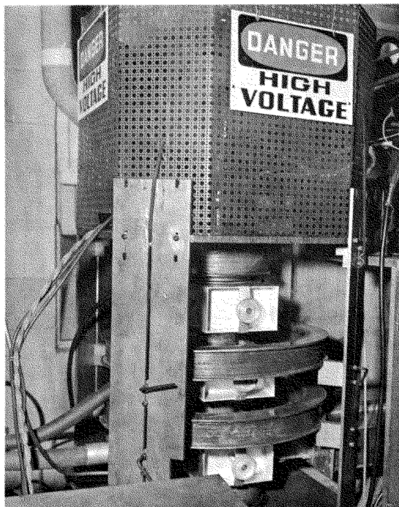
Fig. 8—The 5-kw klystron on test.
