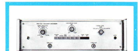
NTSC compact coder PM 5553 incorporates the sub-carrier oscillator.
