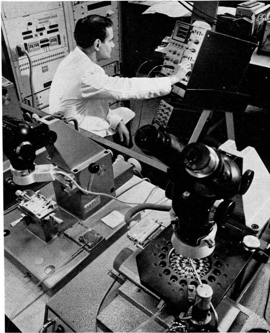
PM 3370 and PM 3372 in use with a computer-controlled set-up for tests and measurements on silicon wafers for integrated circuits
