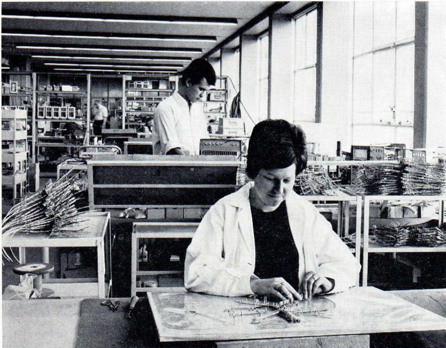
Making the cable form of the PM 3370
