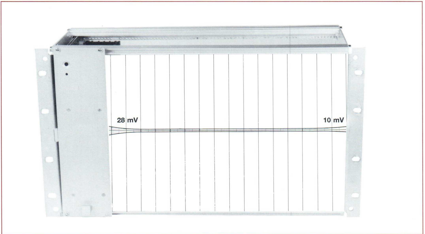
FIG. 22. MEASUREMENTS ON A RACK-MOUNTED PE 1126 (OPEN TYPE)
