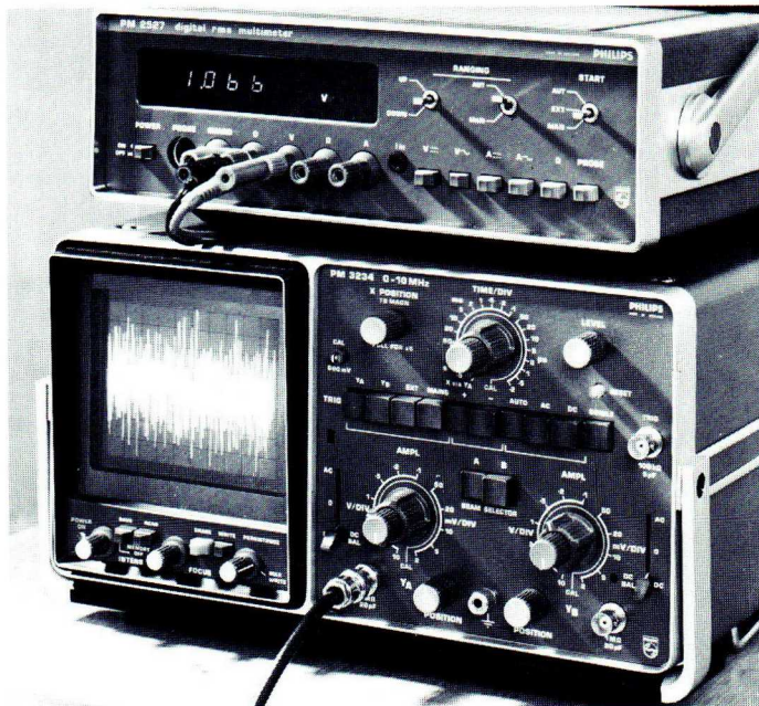
Fig. 7.32. Measuring noise with the PM 2527. The oscilloscope is set to a vertical sensitivity of 1 \text{ V/div}
