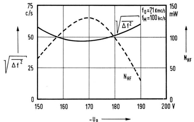
Fig. 12 Noise level and RF energy as a function of reflector voltage
