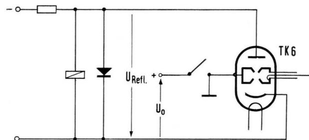
Fig. 15 Proposed circuit for the automatic disconnection of the resonator voltage when there is no, or a positive, reflector voltage
