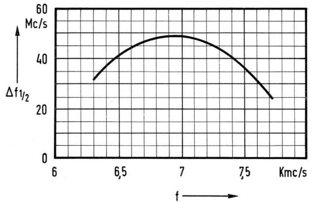
Fig. 8 Electronic bandwidth as a function of frequency
