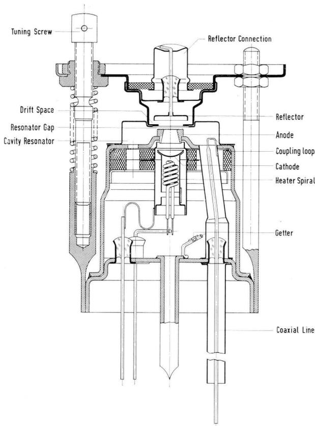
Fig. 2 Design of the Reflex Klystron **TK 6**
