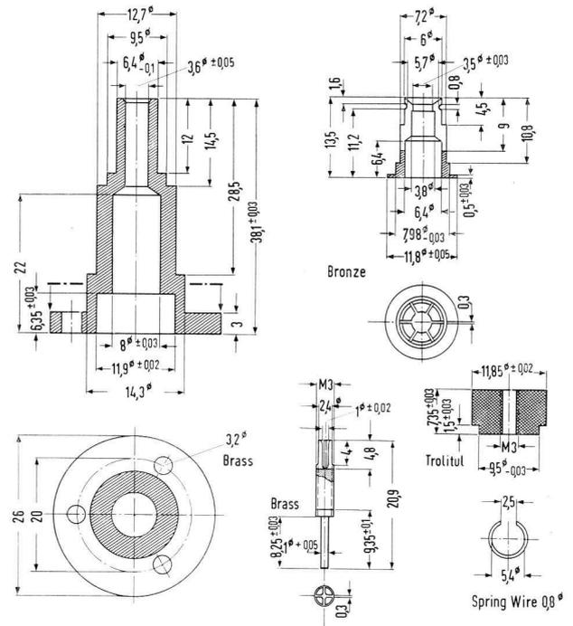
Fig. 5 Components of waveguide coupling
