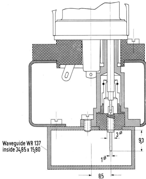
Fig. 4 Example for coupling tube **TK 6** to a square waveguide
