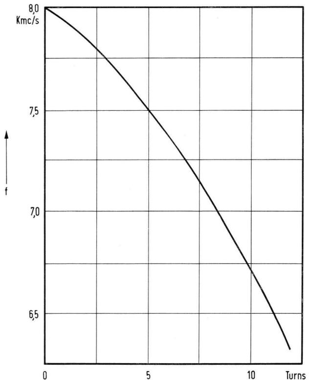
Fig. 3 Klystron frequency as a function of the number of turns of the tuning screw
