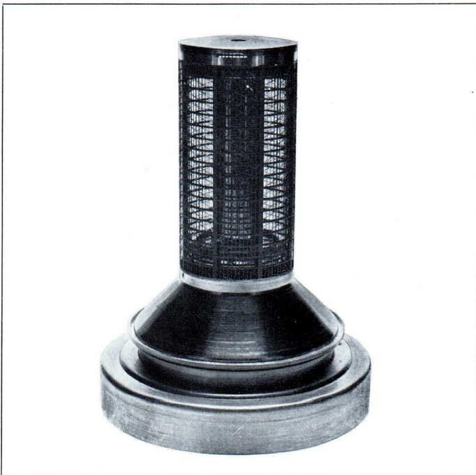
Fig. 1 Grid-cathode structure of the RS 2022 CL
