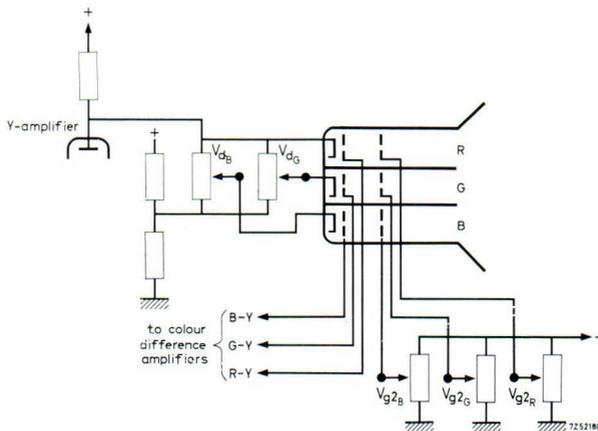
Fig. 16. Driving the picture tube with a “potentiometer” circuit.
