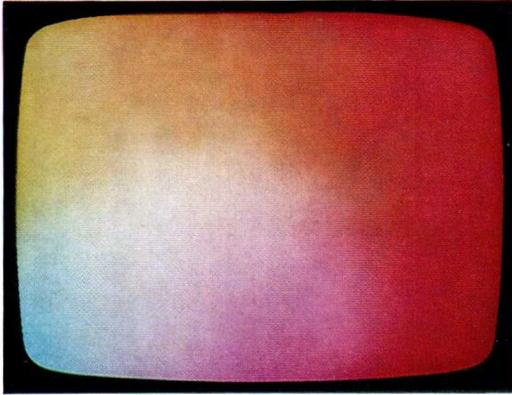
*Fig. 22. Picture with non-adjusted colour purity. Only the red beam is switched on.*
