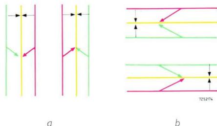
*Fig. 15. Matrixed convergence adjustment of red and green by means of a cross-hatch pattern. (a) Similar shifts of the red and green beam produce a shift of the vertical red and green lines only. (b) Opposite shifts of the red and green beams produce a shift of the horizontal red and green lines only.*
