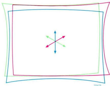
Fig. 10. Typical raster shape without dynamic convergence correction of the convergence errors.
