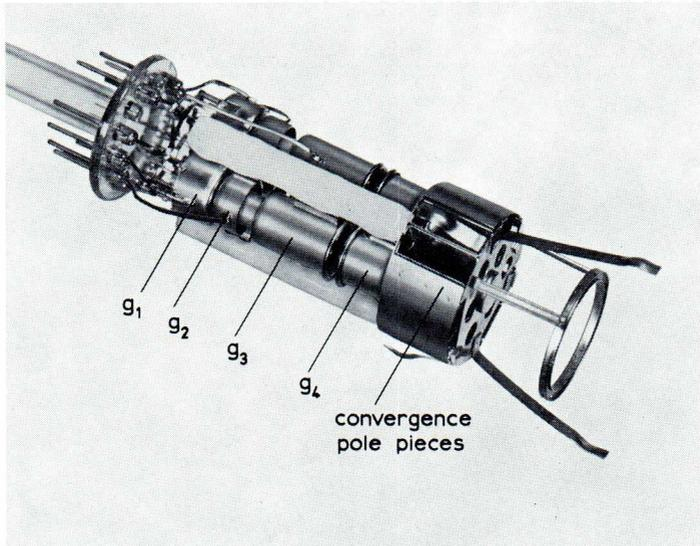
Fig. 6. Electrode system of the A63-11X colour picture tube.
