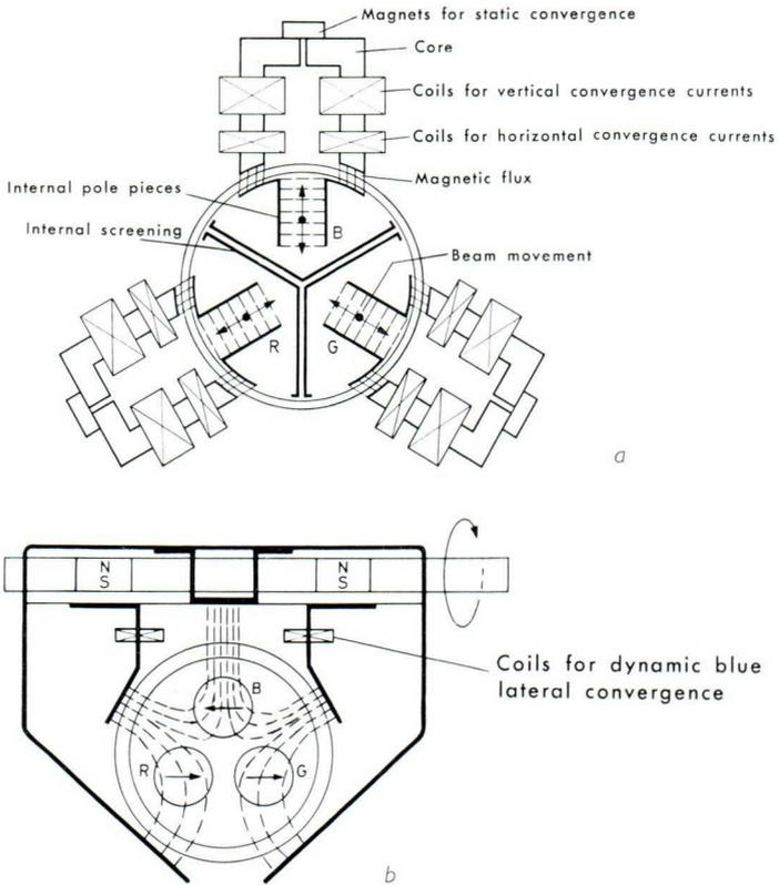
Fig. 3. Convergence adjustment. (a) The magnetic correction fields of the convergence unit act on the three electron beams by means of magnetic pole pieces. (b) The blue lateral shift system acts on the blue beam and, simultaneously, but with opposite effect, on the red and green beams.
