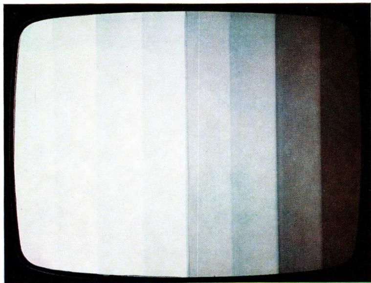
*Fig. 34. Correctly adjusted grey scale in the colour picture tube.*
