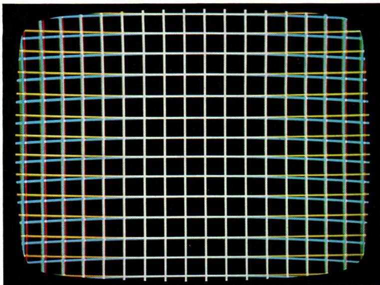
*Fig. 28. Cross-hatch pattern after adjustment of the static and dynamic vertical convergence.*
