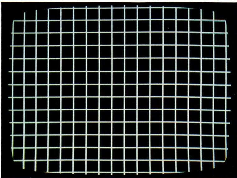
*Fig. 32. Cross-hatch pattern as in Fig. 31, but with raster correction.*
