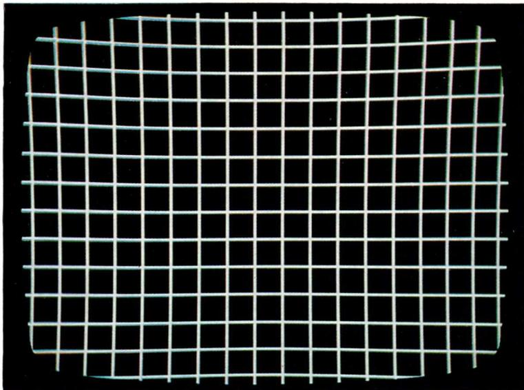
*Fig. 31. Cross-hatch pattern after adjustment of the static and dynamic convergence, without raster correction.*
