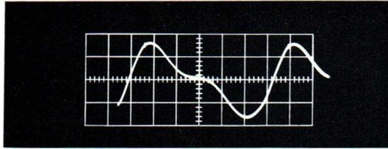
Fig. 29. Voltage across the blue horizontal convergence coil (vertical: 10 V/div, horizontal: 10  $\mu$ s/div).
