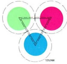
*Fig. 26a. Colour purity adjustment. In the centre of the picture the gravity centres of the two triangles formed by the phosphor triplet and the excited phosphor areas must coincide.*
