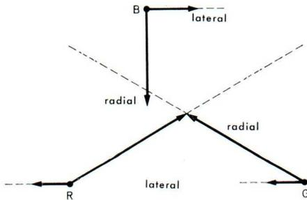
Fig. 7. Directions in which the electron beams can be deflected by the convergence correction fields (seen from the screen).
