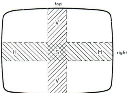
Fig. 19. Area of static (S), dynamic vertical (V) and horizontal (H) convergence adjustment.
