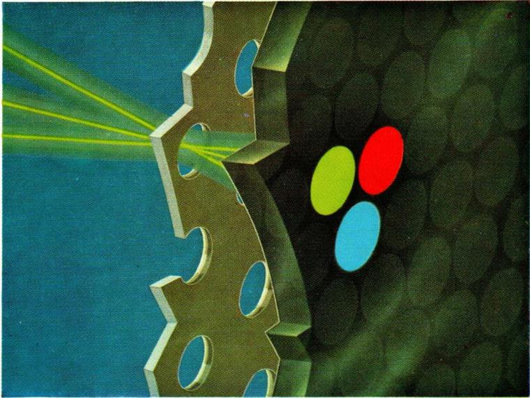
*Fig. 1. Principle of the shadow-mask tube. The angle of incidence of the electron beams on the shadow mask determines which phosphor dots will be excited. In practice, the electron beams will have a larger diameter than the mask holes and will cover several holes simultaneously.*
