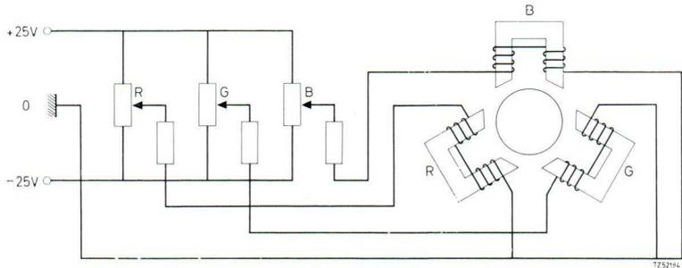
Fig. 8. Example of a circuit for electrical adjustment of the static convergence. The series resistors serve to reduce current variations due to temperature.
