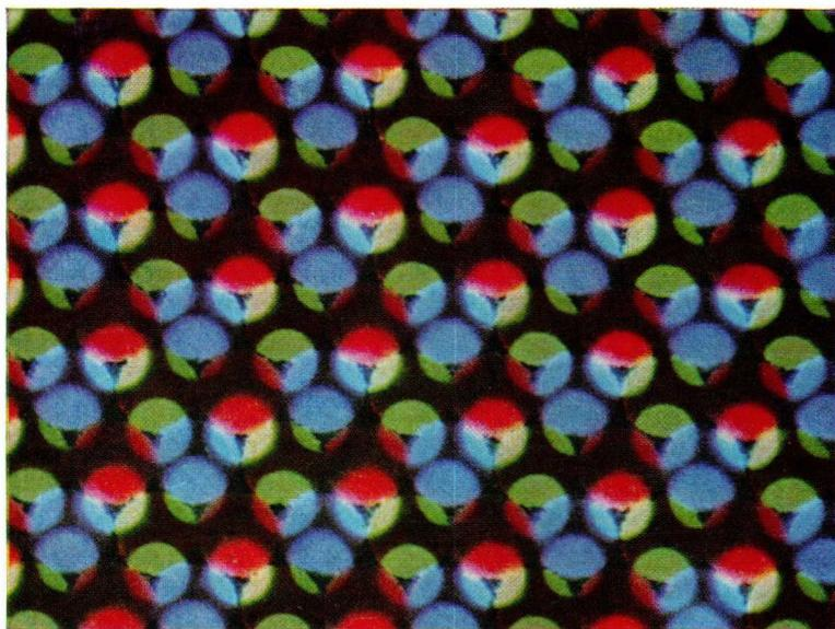
*Fig. 25. Enlarged view of the phosphor screen with mal-adjusted colour purity.*
