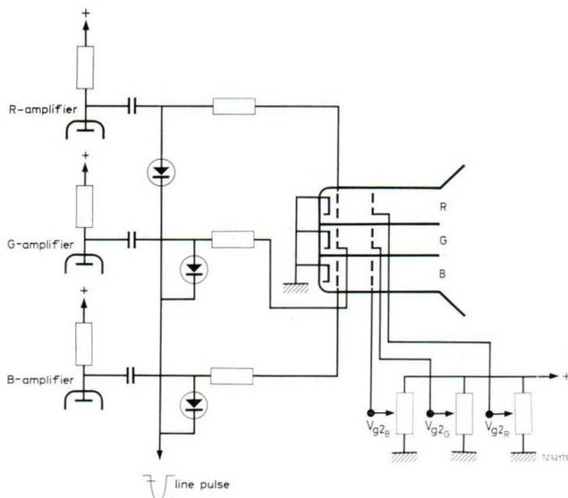
Fig. 17. Driving the picture tube with an RGB drive circuit.
