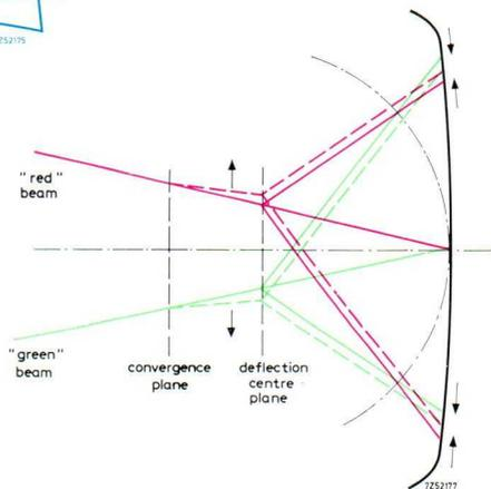
Fig. 11. Correction of dynamic convergence errors by making the eccentricity of the beams at the deflection centre to vary with the scan (shown for the red and green beams only).
