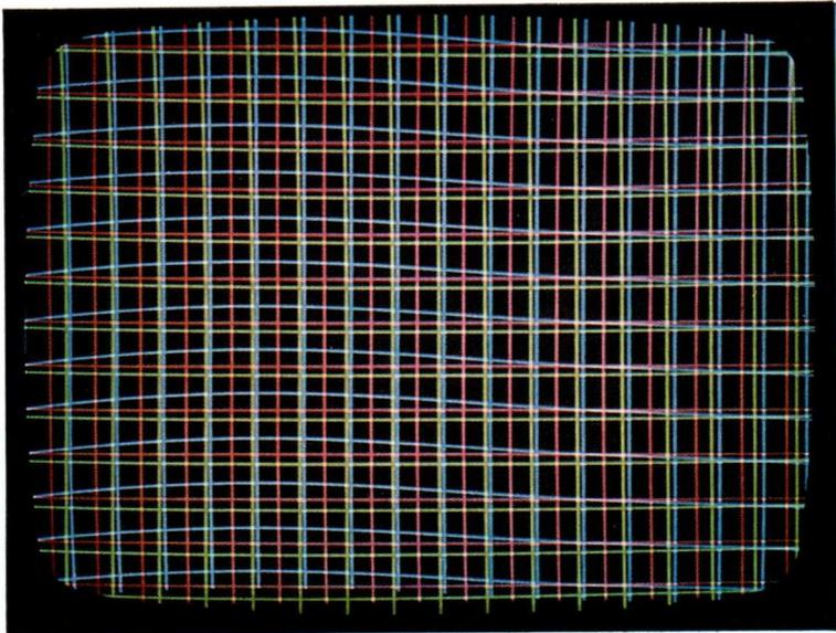
*Fig. 18. Cross-hatch pattern before convergence adjustment. Lack of convergence also gives rise to colour impurity.*
