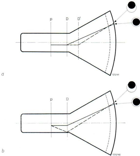
Fig. 4. (a) Path of an electron beam with incorrectly (broken line) and correctly (continuous line) adjusted deflection coil. (b) Path of an electron beam with incorrectly (broken line) and correctly (continuous line) adjusted colour purity magnet.
