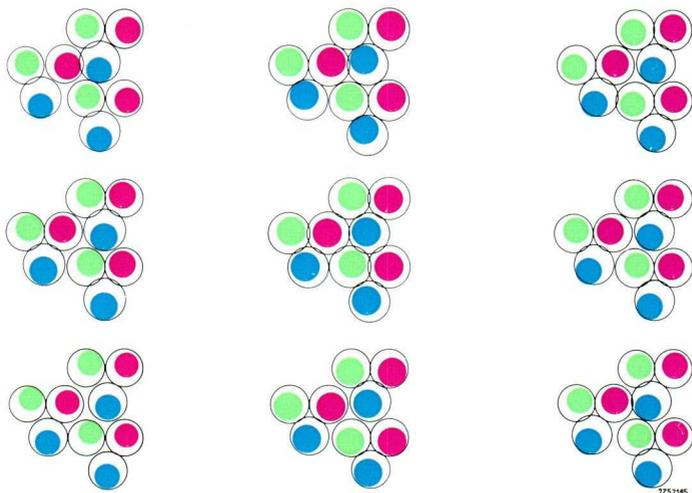
*Fig. 27. Average landing pattern of an A63-11X colour picture tube with deflection coil AT1022/03. The picture shows the landing at the corners of the screen and in the intermediary areas.*
