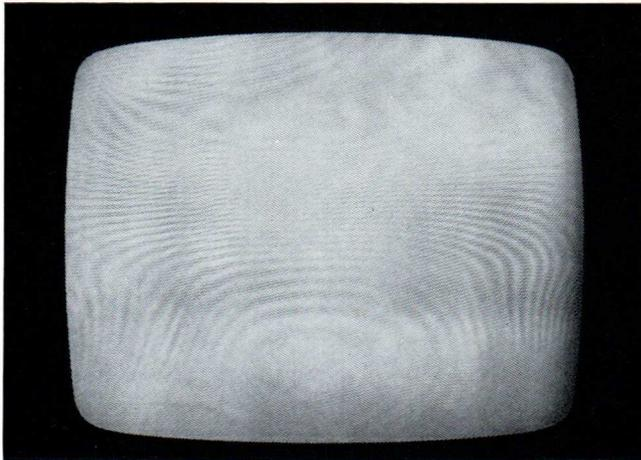
*Fig. 36. Moiré effect as may occur in dark parts of the picture when focusing is adjusted at too low a beam current.*
