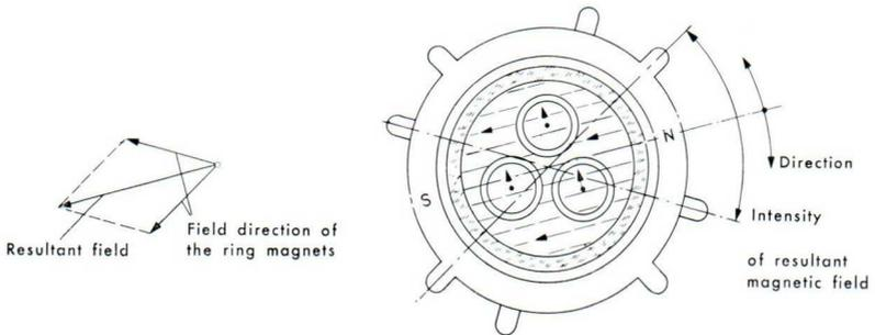
Fig. 5. The colour purity is adjustable by means of two rotatable, magnetised rings.
