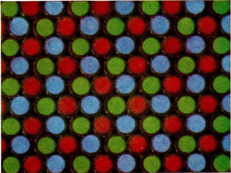
*Fig. 26b. Enlarged view of the centre of the screen with properly adjusted colour purity.*
