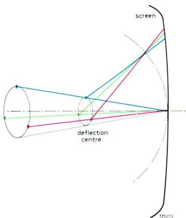
Fig. 9. The flatness of the screen causes dynamic convergence errors. The imaginary cone of which the three beams can be thought of as being parts, is not "focused" at the edges of the screen.
