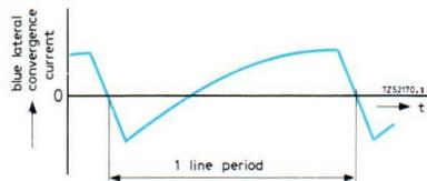
Fig. 12. Convergence errors at the screen axes, and the currents required for correction.
