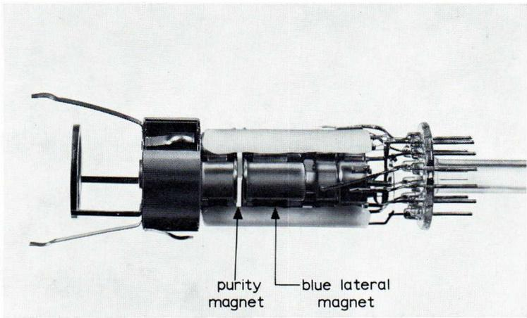
Fig. 2. Position of the deflection and correction systems on the neck of a colour picture tube. The colour purity magnet should be positioned over the gap between grids  $g_3$  and  $g_4$ ; the location of the blue lateral shift system is above the centre of  $g_3$  (the focus electrode).
