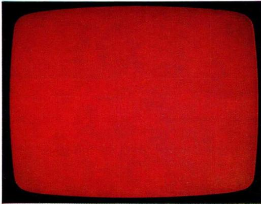
*Fig. 23. Properly adjusted colour purity of the red raster.*
