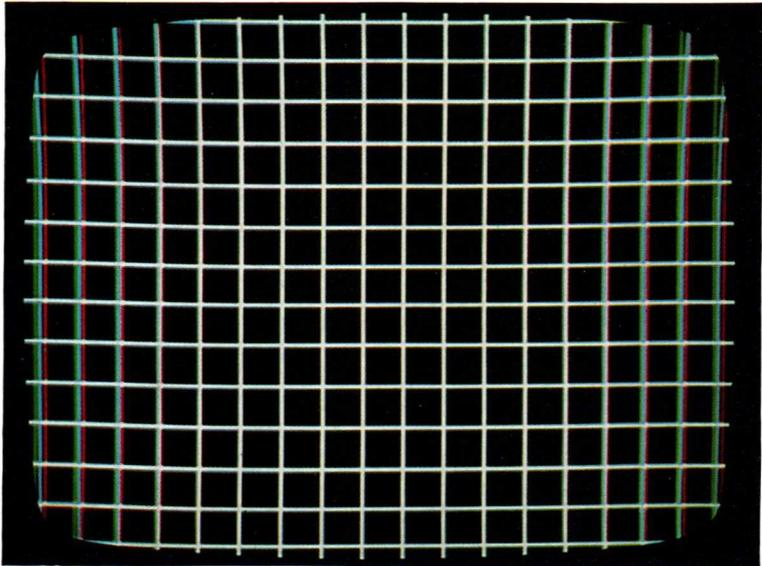
Fig. 30. Cross-hatch pattern after adjustment of the complete radial convergence, but without dynamic blue lateral convergence.
