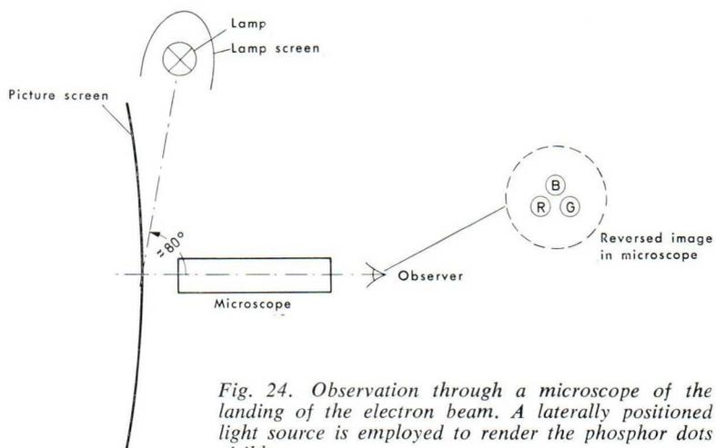
*Fig. 24. Observation through a microscope of the landing of the electron beam. A laterally positioned light source is employed to render the phosphor dots visible.*
