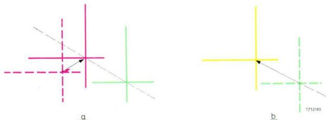
Fig. 20. Static convergence adjustment. (a) Shift of the red grid. (b) Shift of the green grid.
