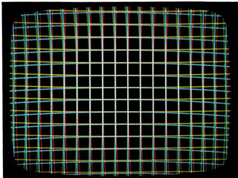
*Fig. 21. Cross-hatch pattern after adjustment of the static convergence.*
