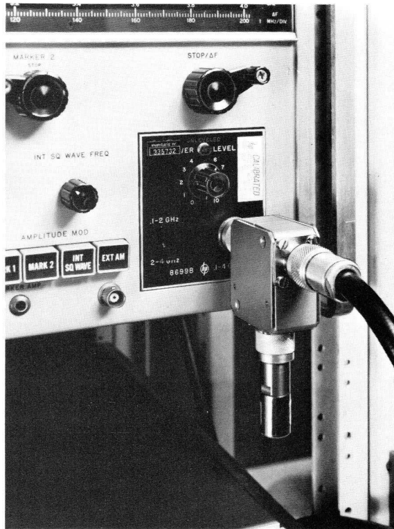
Fig. 23 An example of the use of an isolator (isolator-connected circulator) in a measurement facility. An isolator should always be sited close to the equipment with which it is associated.
