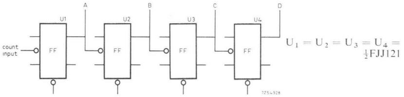
Fig. 77. Asynchronous binary "up counter".
