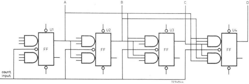
Fig. 79. Synchronous binary "up counter".
