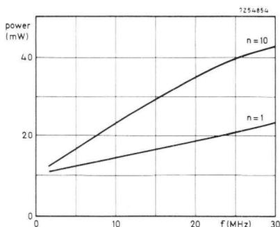
Fig. 11. Typical variation in dissipation with loading and frequency.
