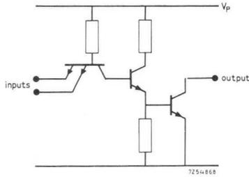
Fig. 30. One section of the FJH231.
