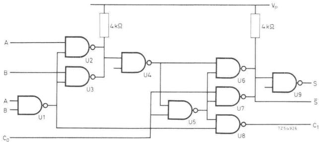
Fig. 74. Full adder using NAND gates.
