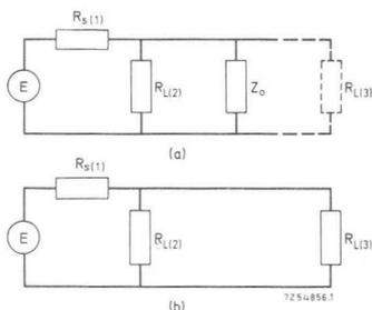
Fig. 13. Equivalent circuit of transmission line connection of gates: (a) during switching transient; (b) under static conditions.
