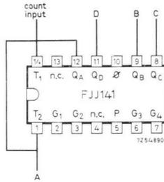
Fig. 101. The FJJ141 element connected as a 1248BCD decade counter.
