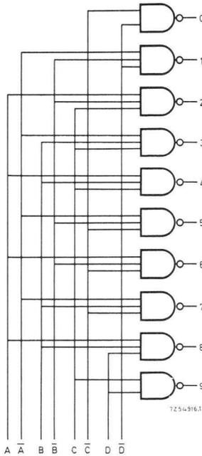
Fig. 54. Excess-three code to decimal converter.
