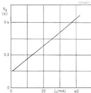
Fig. 7. Typical output characteristic of a TTL gate in the LOW state.
