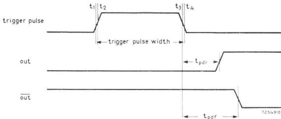
Fig. 33. Operation of master-slave bistable element with  $J = \text{HIGH}$  and  $K = \text{LOW}$ .
