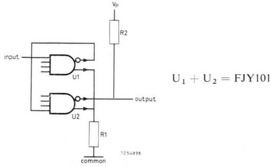
Fig. 120. Level detector using FJY101.
