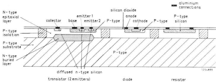
Fig. 1. Cross-section through part of a silicon chip.
