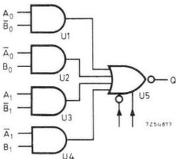
$$Q = \overline{A_0 \cdot \bar{B}_0 + \bar{A}_0 \cdot B_0 + A_1 \cdot \bar{B}_1 + \bar{A}_1 \cdot B_1} = (A_0 \cdot B_0 + \bar{A}_0 \cdot \bar{B}_0)(A_1 \cdot B_1 + \bar{A}_1 \cdot \bar{B}_1)$$
