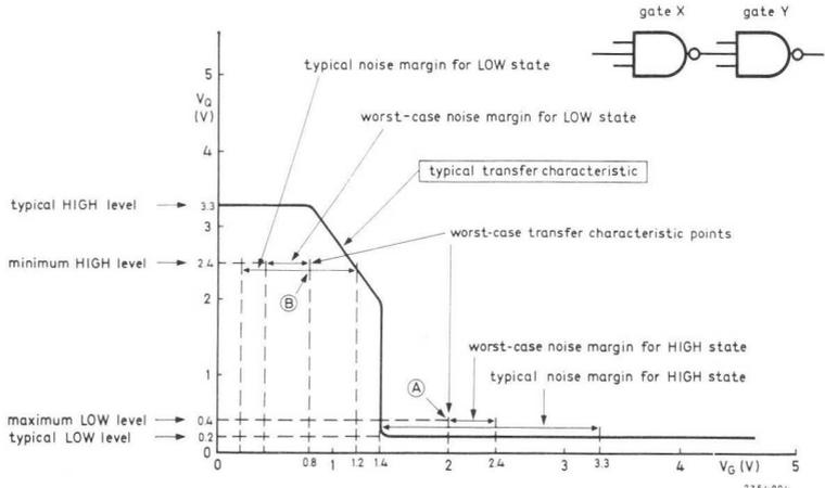
Fig. 10. Typical transfer characteristic of a TTL gate.
