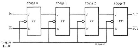
Fig. 21. Shift register using J-K bistable elements.
