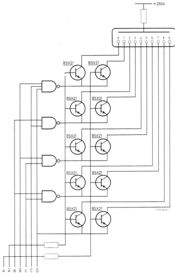
Fig. 52. 1248BCD to decimal converter and numerical indicator tube driver.
