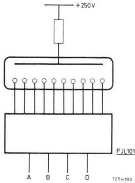
Fig. 53. 1248BCD to decimal converter and numerical indicator tube driver using FJL101.
