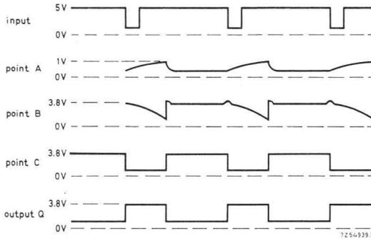
Fig. 116. Waveforms for three-gate monostable circuits.
