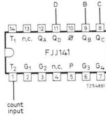
Fig. 102. The FJJ141 element used as a modulo-5 counter.
