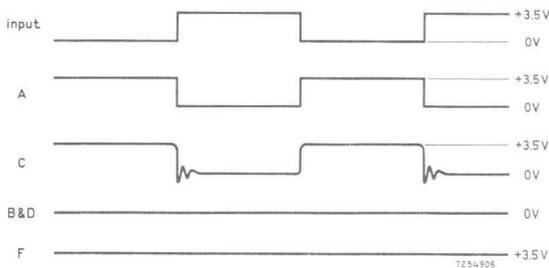
Fig. 16. Waveforms obtained with switch  $S_1$  of Fig. 15 open.
