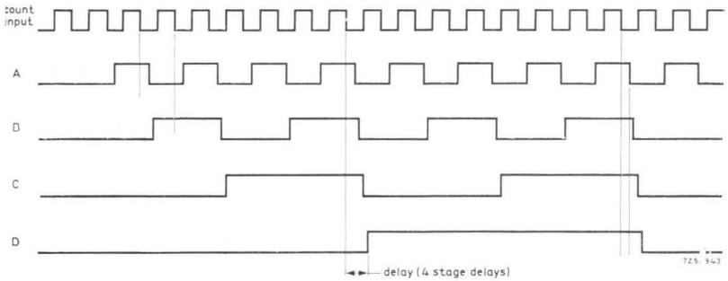
Fig. 78. Waveforms for asynchronous binary "up counter".
