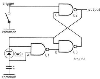
Fig. 114. Three-gate monostable circuit without triggering circuit.
