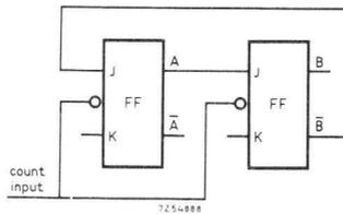
Fig. 84. Synchronous modulo-3 “up counter”.
