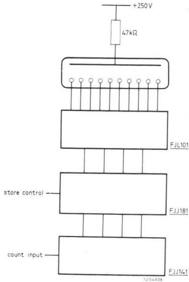
Fig. 113. Block diagram illustrating use of quadruple D bistable element FJJ181 as gated staticiser in conjunction with a decade counter and a numerical indicator tube driver.
