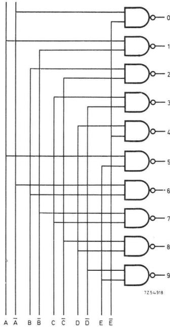
Fig. 56. Johnson code to decimal converter.
