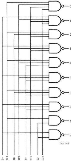
Fig. 51. 1248BCD to decimal converter.
