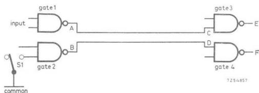
Fig. 15. Gates connected by twin pair.
