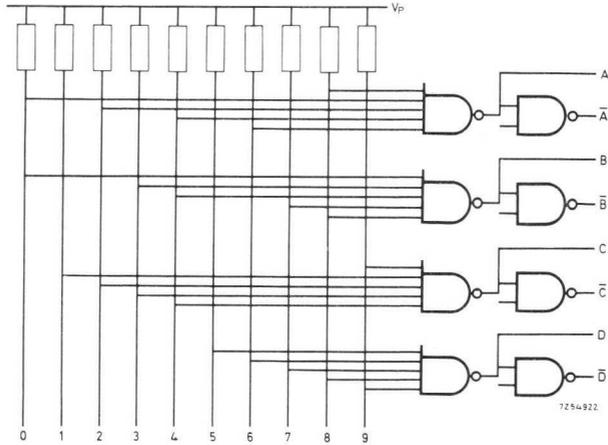
Fig. 60. Decimal to excess-three code converter.
