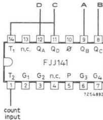
Fig. 103. The FJJ141 connected as a divide-by-ten counter counting in 1245BCD.
