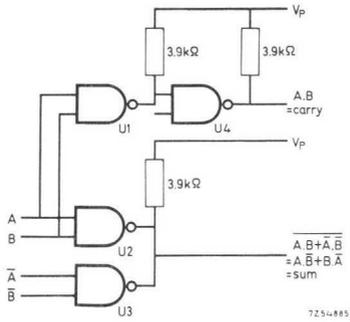
Fig. 70. Half adder using one FJH231.
