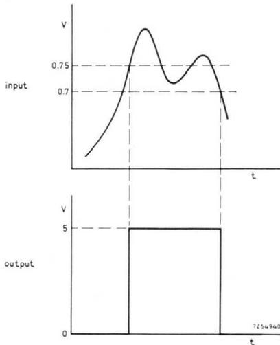
Fig. 121. Performance of level detector with values of  $R_1$  and  $R_2$  of  $56 \Omega$  and  $3.3 \text{ k}\Omega$  respectively, and a fan-out of 1.
