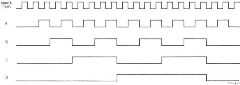
Fig. 80. Waveforms for synchronous binary "up counter".
