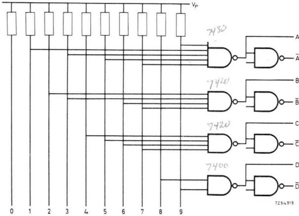
Fig. 57. Decimal to 1248BCD converter.
