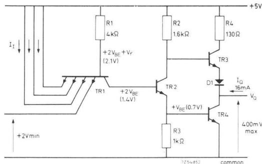
Fig. 6. TTL gate showing the conditions with all inputs HIGH.
