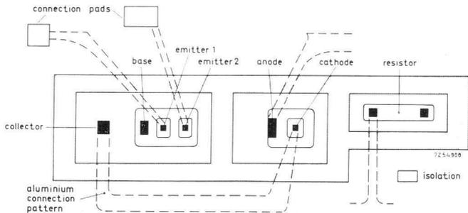
Fig. 2. Plan view of a silicon chip.
