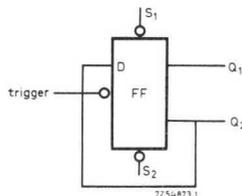
Fig. 35. D bistable element connected as a T bistable element.
