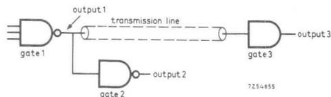
Fig. 12. Gates connected by a long transmission line.
