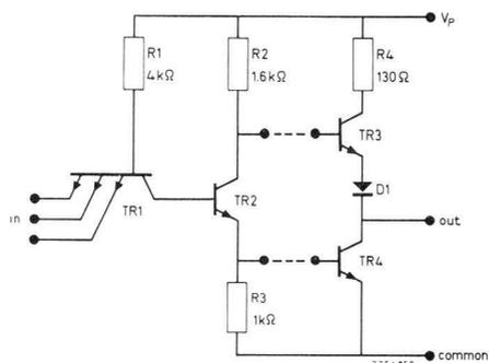
Fig. 4. TTL gate and output stage.
