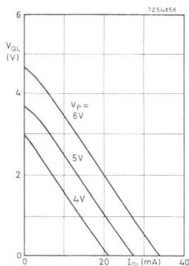
Fig. 18. Typical variation in output characteristic with variation in supply voltage in the HIGH state.
