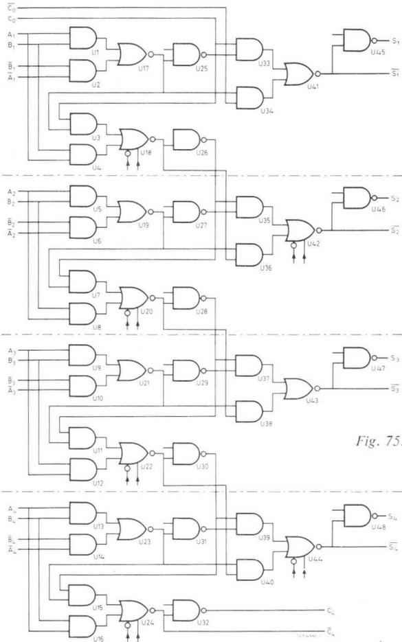
Fig. 75. Four-bit binary adder.
