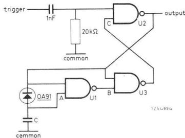
Fig. 115. Three-gate monostable circuit with triggering circuit.
