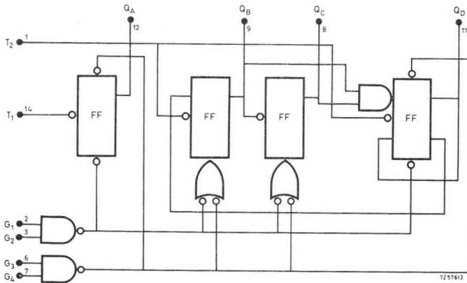
Fig. 100. Circuit diagram of FJJ141 element.
