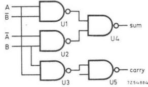
Fig. 69. Half adder using one FJH131.
