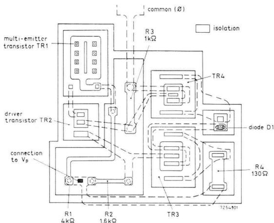
Fig. 3. TTL gate on a silicon chip.
