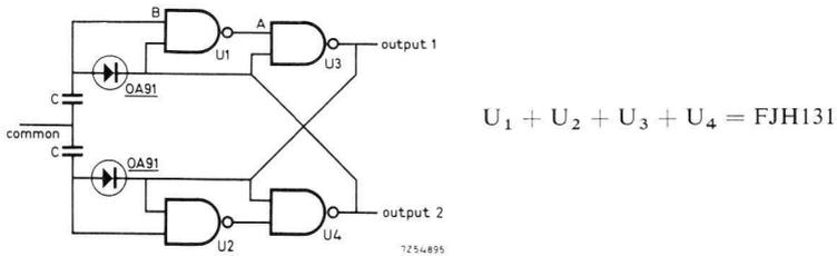
Fig. 117. Four-gate multivibrator.
