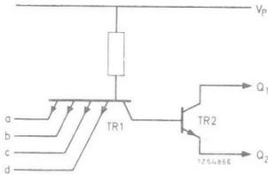
Terminals  $Q_1$  and  $Q_2$  are to be connected to inputs  $E_1$  and  $E_2$  respectively, of FJH151 or FJH171; suggested resistor value  $4\text{ k}\Omega$ .
