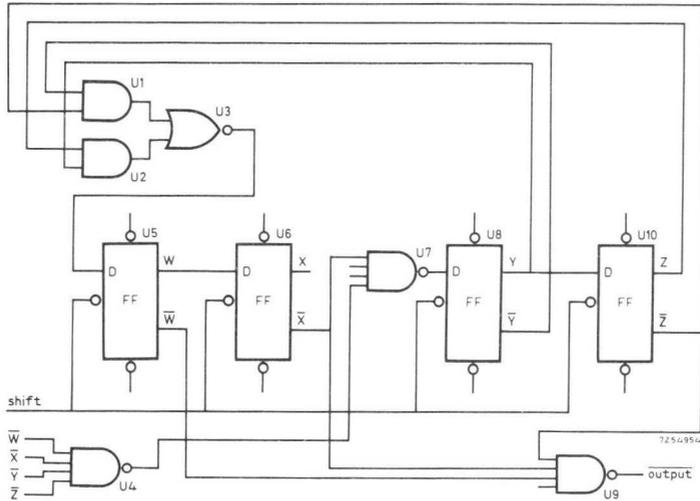
Fig. 106. Four-stage chain code generator with cycle length of fifteen.
