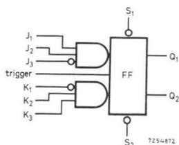
Fig. 34. Edge-triggered J-K bistable element type FJJ101.
