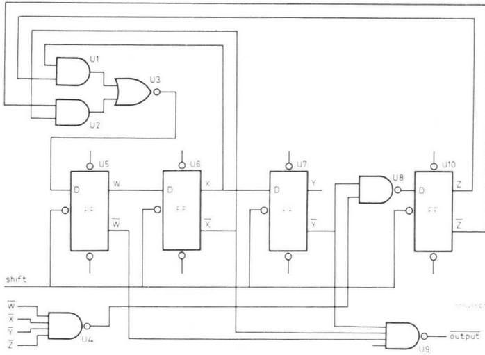
Fig. 108. Example of a chain code generator with cycle length of less than  $2^n - 1$ .
