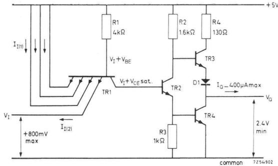
Fig. 8. TTL gate showing the conditions in the OFF state.
