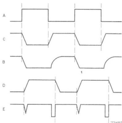
Fig. 25. Waveforms illustrating severe transient hazards.
