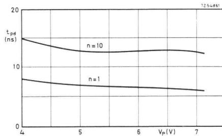
Fig. 20. Variation in propagation delay with variation in supply voltage.
