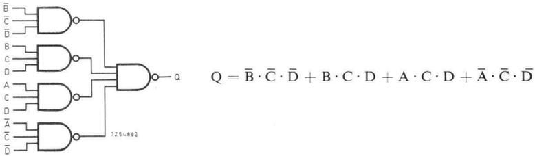
Fig. 66. Excess-three code error detector.
