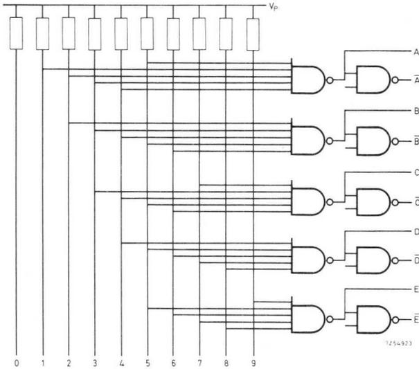
Fig. 61. Decimal to Johnson code converter.
