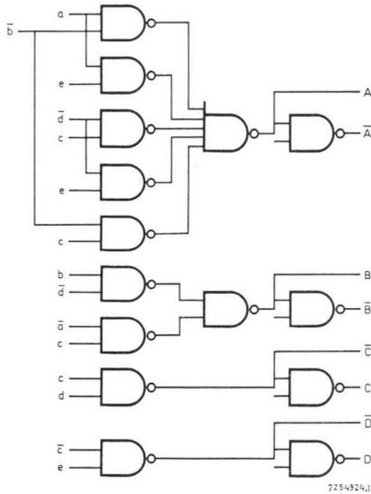
Fig. 62. Johnson code to 1248BCD converter.
