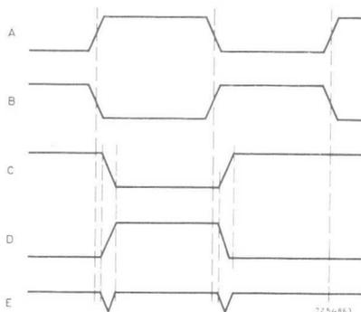
Fig. 23. Waveforms illustrating transient hazards.
