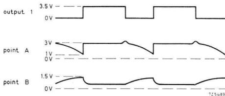
Fig. 118. Waveforms for four-gate multivibrator with a value of  $C$  of 100 nF.
