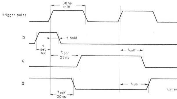
Fig. 36. Waveforms of *D* bistable element FJJ131.
