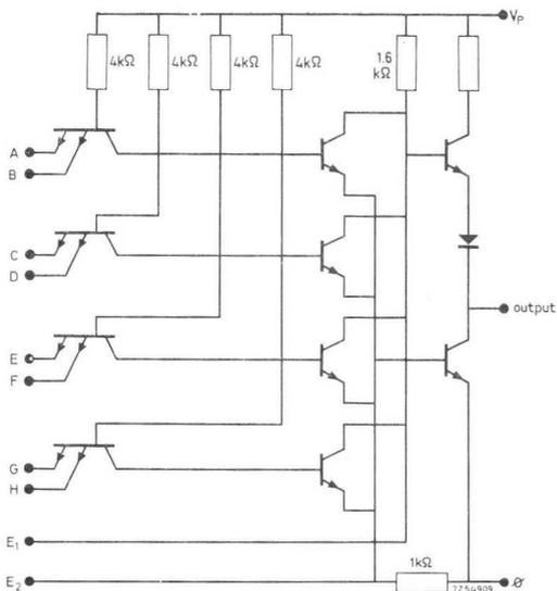
Fig. 29. Circuit diagram of the quadruple AND-OR-NOT gate type FJH171.
