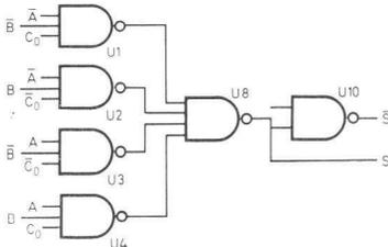
Fig. 73. Full adder using NAND gates.
