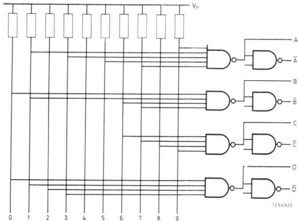
Fig. 58. Decimal to 1242BCD converter.
