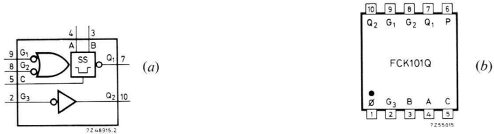
Fig. 2-61. The Monostable Multivibrator, FCK101Q (without extra gate facility). (a) Block diagram; (b) pin layout and numbering.
