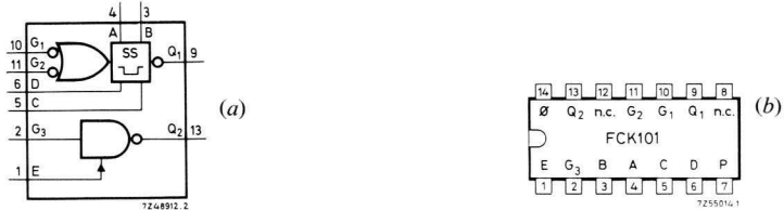
Fig. 2-62. The Monostable Multivibrator, FCK101 (with extra gate facility). (a) Block diagram; (b) pin layout and numbering.
