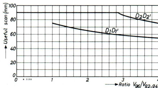
Fig.3. Useful scan plotted against the ratio V_{g6}/V_{g2,g4}
