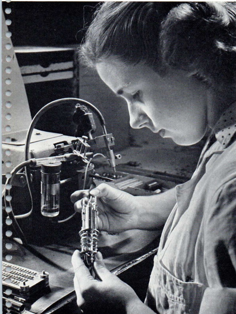
Supports for the heater-cathode assembly are aligned with tweezers. To produce clean and sturdy joints welding is done in an atmosphere of inert gas.
