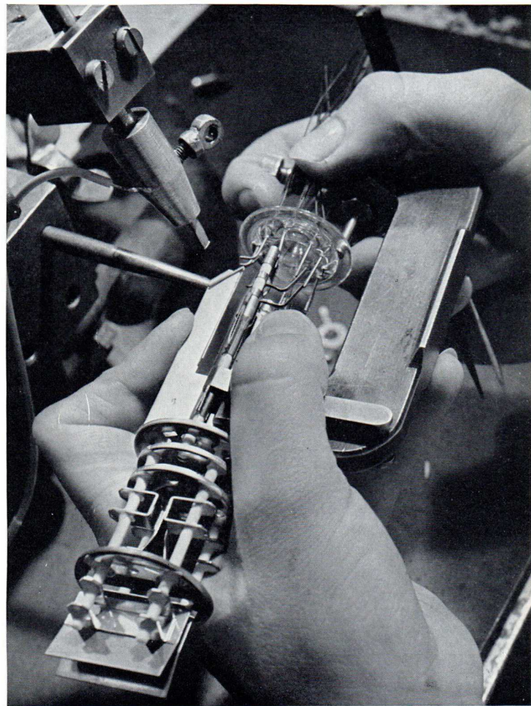
The electrode assembly is welded to the lead-in wires.
