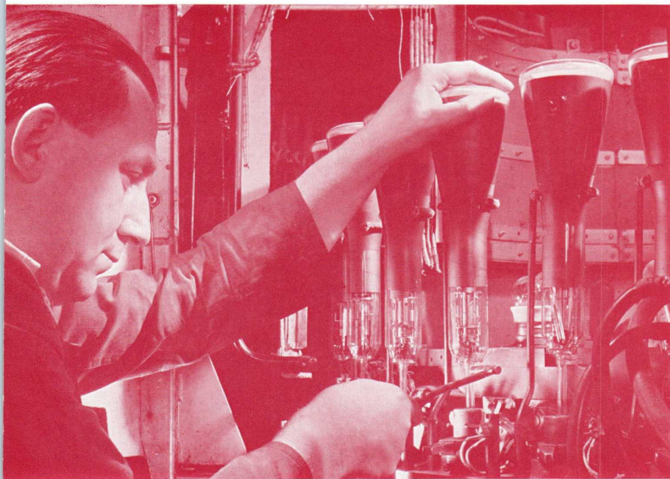
Pumping and sealing off is done on an intricate automatic machine. During the pumping process the tubes pass through several phases of normal and high-frequency heating to remove the last traces of gas.
