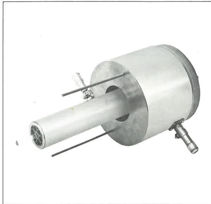
Figure 14. End view of cavity. Coaxial input receptacle is at left on cathode line. The two plate tuning rods project from the bottom of the cavity. The cathode tuning rod projects from the end of the air filter at left. A sectional view of the rf filter is shown in Fig.15.
