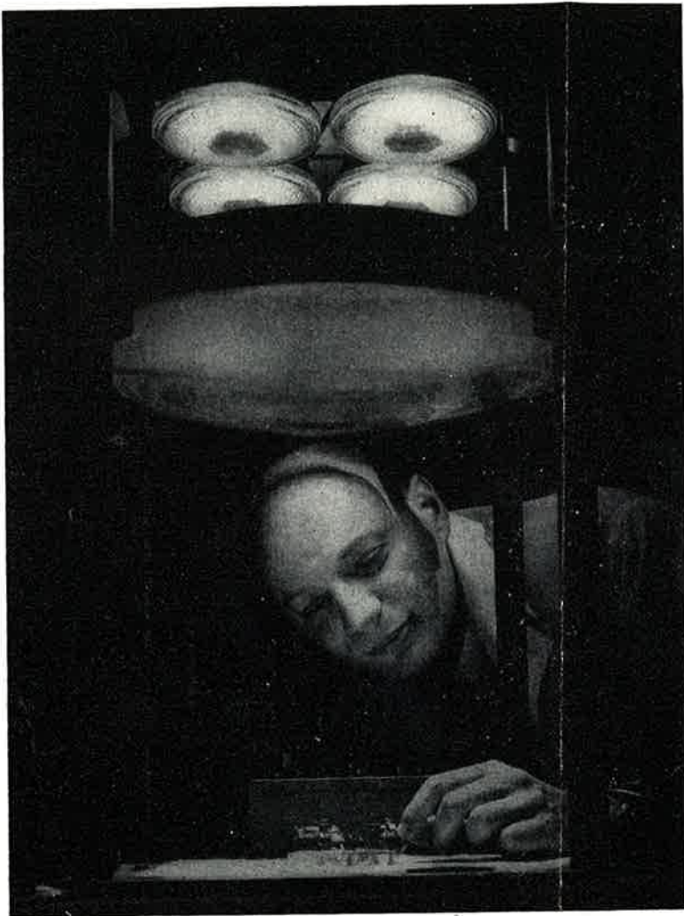
Paul Rappaport, RCA Laboratories technical staff, tests solar cell power output under a simulated solar source.
