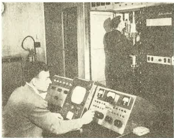
Fig. 7.—Control Console and Cavity Resonators at Station KC2XAK.
