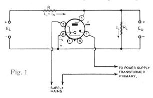
If  $R_{\rm L}$  is a load of varying resistance, or if the whole device be regarded as a source of approximately constant voltage for any load, the minimum value of R may readily be calculated. If there is no load current (i.e.,  $R_{\rm L}$  is open circuited), the whole current must pass through the tube and is therefore limited to 30 mA.
