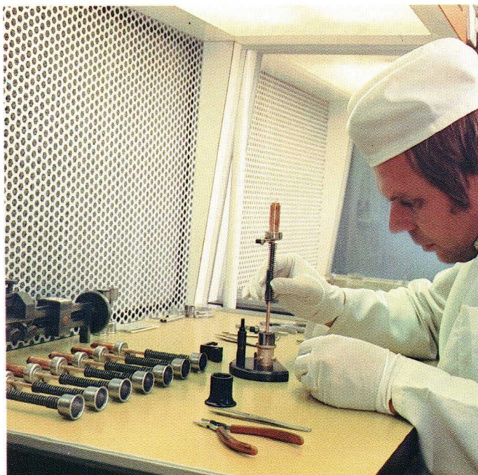
3 3 Series production of radio-link TWT's. These tubes are awaiting assembly of the PPM magnets.
