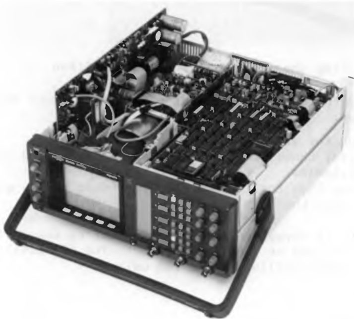
Figure 16.2 Power supply unit in service position.
